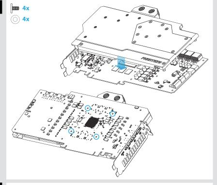
Make sure to lay the GPU with the water block flat down without resting on the PCI bracket.
