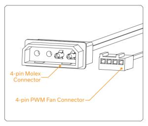
The EK-D5 PWM pump has two connectors.
