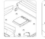
Remove motherboard stock plastic brackets, keep the stock backplate, put AM4 plastic spacers onto backplate screw threads. Then fix both brackets on spacers using AMD screws.
