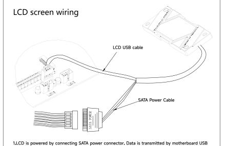
connector. Please confirm proper connection before software install. 2.Download TRCC at: https://www.thermalright.com/support/download/ Unzip setup file and start install by double click setup. 3. After install completed, double click shortcut icon on desktop to run software. 4.All functions on LCD are controlled by software, and software will auto start at OS boot. Please
