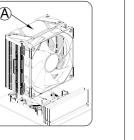
Apply thermal paste on CPU IHS, put heatsink onto the CPU and align both nuts to screw threads on brackets. Gently tighten both nuts with screw driver to mount heatsink on CPU.
