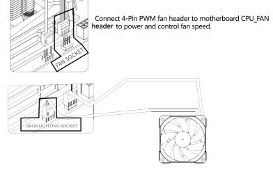
For Fans with Addressable-RGB lighting, connect 3-Pin ARGB lighting header to motherboard 3-Pin +5V ARGB lighting header to control
