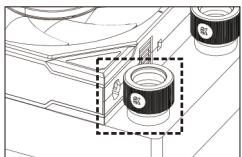
**Note!** If the radiator outlet affects the fan interlocking key, you can remove them/若遇到水冷排出水位置影響風扇扣鎖，可將風扇卡扣鎖移除/
