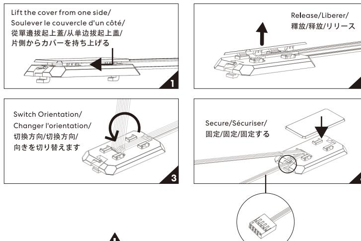
It is recommended to secure the clip at the USB connector to help the top cover stay in place/
