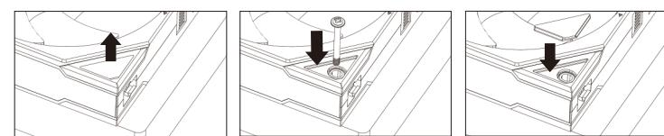
Secure the fan to the radiator and cover with the rubber pads to enhance the overall aesthetics/
