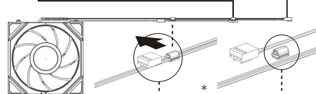
\* The plastic cable clip has a large and small side/
