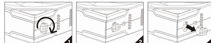
**!** If the radiator outlet interferes with the fan interlocking key, you can remove them/
