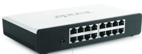
Side Vent Bottom Vent 94V0 Fireproof Plastic Housing
