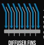
The angular fins largely extend the contact surface of the air and the fins, enabling the air current to transmit in the steadiest way.
