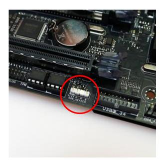
• 1) Require motherboard with ARGB header to enable ARGB lighting
