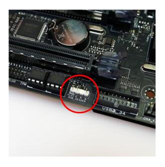
• 1) Require motherboard with ARGB header to enable RGB lighting
