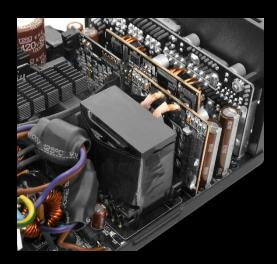
High Amperage Single +12V Rail & DC to DC Design
